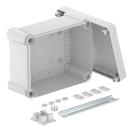
Junction box with hat profile rail for the connection of cables and lines indoors and in outdoor areas. Rectangular design without entries. Suitable for wall and ceiling mounting with the option to fasten outside, inside or to mount via the corner domes. Particularly impact resistant with IK09. Cover with quick lock, sealable. Made from halogen-free and UV-resistant materials.
