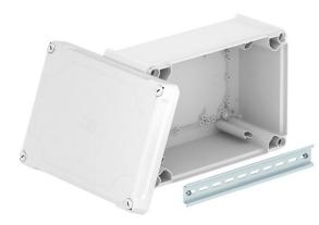
Closed junction box for the connection of cables and lines indoors and in protected outdoor areas. Rectangular design without entries. Suitable for wall and ceiling mounting, on mounting panels and threads in the floor. With the option to fasten inside and to mount via the corner domes. High, transparent cover with quick lock, sealable. Made from halogen-free and UV-resistant materials.
