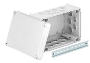
Junction box for the connection of cables and lines indoors and in protected outdoor areas. Rectangular design with plug-in seals. Suitable for wall and ceiling mounting, on mounting panels and threads in the floor. With the option to fasten inside and to mount via the corner domes. High, transparent cover with quick lock, sealable. Made from halogen-free and UV-resistant materials.
