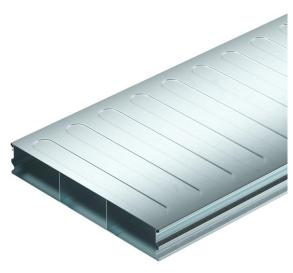
Underfloor trunking (2 piece) for routing cables in screed-covered underfloor systems, according to EN 50085-2-2. Removable and continuously lockable trunking cover. With separating retainers in the trunking base. Maximum load-bearing capacity to 1.5 kN. Only compatible with the UZD250-4/350-4
