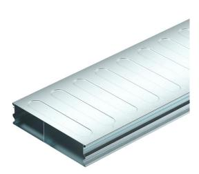
Underfloor trunking (2 piece) for routing cables in screed-covered underfloor systems, according to EN 50085-2-2. Removable and continuously lockable trunking cover. With separating retainers in the trunking base. Maximum load-bearing capacity to 1.5 kN. Only compatible with the UZD250-4/350-4
